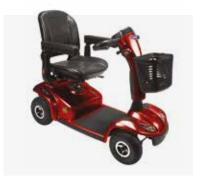
Invacare Leo Max weight capacity: 136kg Max speed: 4mph Max range\*: 22 miles
